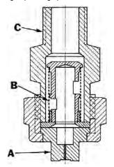
FIGURE 8. Low Pressure Flat Fan Spray Nozzles Used with Special Drop Boom: (A) Nozzle Tip, (B) Strainer, (C) Nozzle Body.
