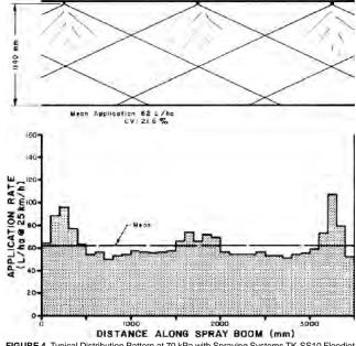
FIGURE 4. Typical Distribution Pattern at 70 kPa with Spraying Systems TK-SS10 Floodjet Nozzles, at a 1140 mm Nozzle Height.
