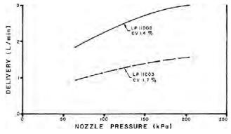
FIGURE 13. Delivery Rates for LP 11003 and LP 11006 Nozzles.
