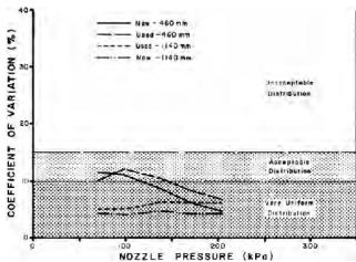
FIGURE 12. Spray Pattern Uniformity for New and Used LP TeeJet 11006 Brass Nozzles, Operated at Heights of 460 and 1140 mm.
