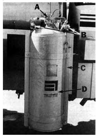
FIGURE 19. Foam Marker Assembly: (A) Refill Valve, (B) Solenoid Valves, (C) Fluid Level Indicator, (D) Foam Tank.
