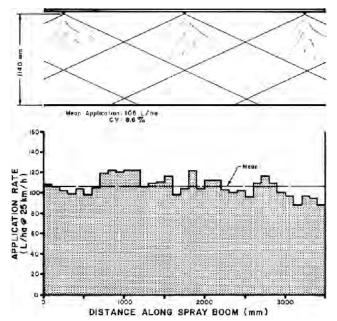
FIGURE 5. Typical Distribution Pattern at 205 kPa with Spraying Systems TK-SS10 Floodjet Nozzles, at a 1140 mm Nozzle Height.
