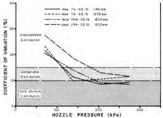
FIGURE 6. Spray Pattern Uniformity for New TK-SS10 Floodjet Nozzles, Operated at 1140 and 1270 mm Nozzle Height and for New and Used 1/4K-SS15. Floodjet Nozzles, Operated at 1270 mm Nozzle Height.
