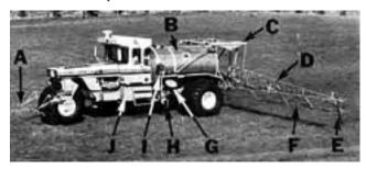
FIGURE 1. Terra-gator 1603 with Liquid System: (A) Front Drop Boom, (B) Spray Tank, (C) Boom Support Members, (D) Main Boom, (E) Foam Marker Drop Hose, (F) Rear Drop Boom, (G) Inductor System, (H) Pump Reload Hose, (I) Flow Meter\*, (J) Fuel Tank.
