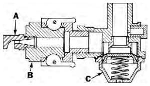
FIGURE 3. Floodjet Nozzle Used with Regular High Clearance Boom: (A) Nozzle, (B) Quick Coupler, (C) Diaphragm Check Valve.
