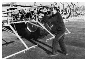
FIGURE 22. Drop Boom Height Adjustment.
